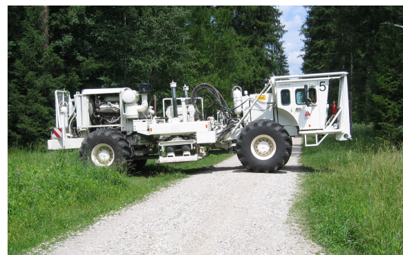
Figure 9: Vibrator used for VSP field experiment.
