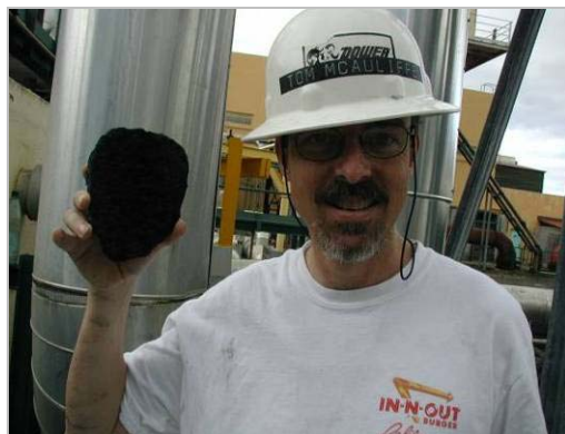
Figure 1. In this photograph taken at Bouillante II in the West Indies, Tom McAuliffe holds a lump of mineral scale removed from plant equipment. The potential for scaling is one of the design challenges that set geothermal plants apart from more conventional plants.
