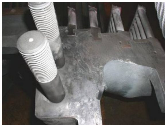
Figure 7: Corrosion and erosion at the diaphragm holder face joint
