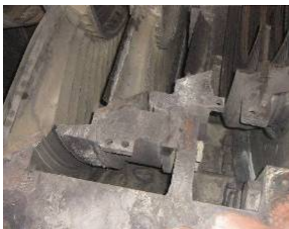
Figure 8: Corrosion at Unit 1 LP stationary blade ring
