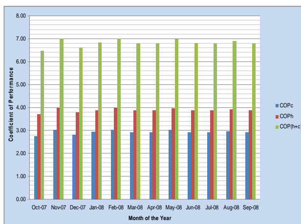
Figure 7: COPs Based on CHW and LGHW Temperatures (Oct 2007 – Sept. 2008)
