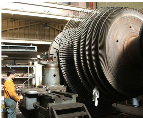
Figure 4 - Turbine rectification lathe. 2009 Machining off blade row LP7, of an MP machine rotor at about 3rpm, in preparation for reblading. Lathe operator is behind the rotor. Rag on rotor signals to assistant when to increment the tool post.
