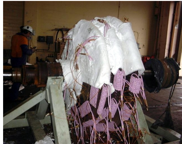
Figure 5 - Rotor heat treatment post weld repairs to remedy tenon erosion.
