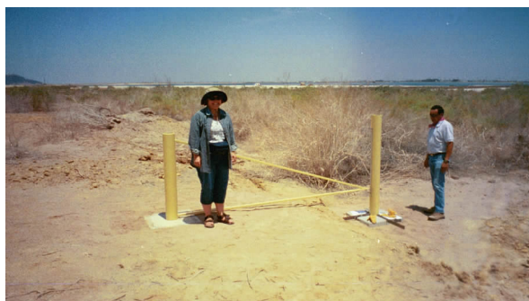
Figure 3. 3-D Witness installed over the Cerro Prieto fault in 2004 at point F2 (Fig.1).
