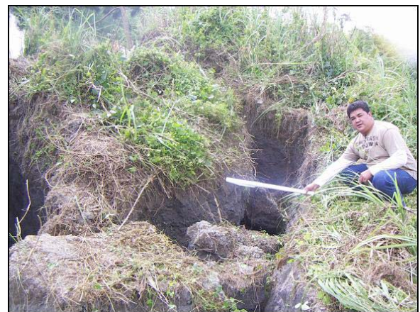
Figure 8. Cracks noted within the bedrock at the base of the slide.
