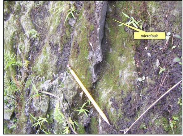
Figure 11. Photo shows recent microfault displacement on a bedrock near the base of the slide.
