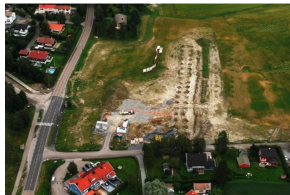
Figure 3: The BTES at Ahus under construction in summer 2007 (Photo: Forum Fjernvarme).
