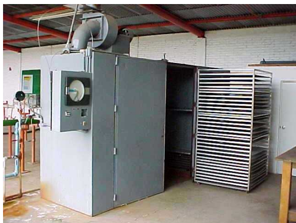
Figure 4: Fruits and vegetables dehydrator prototype constructed by CFE in Los Azufres.
