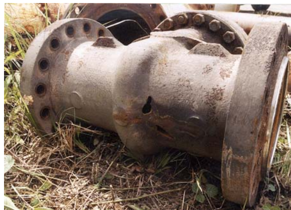
Figure 1. Well 413D sacrificial valve damaged by solids carry-over in steam.
