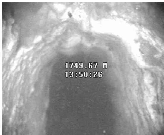
Figure 4: Anhydrite scale at 1,750m pictured by Down Hole Video tool
