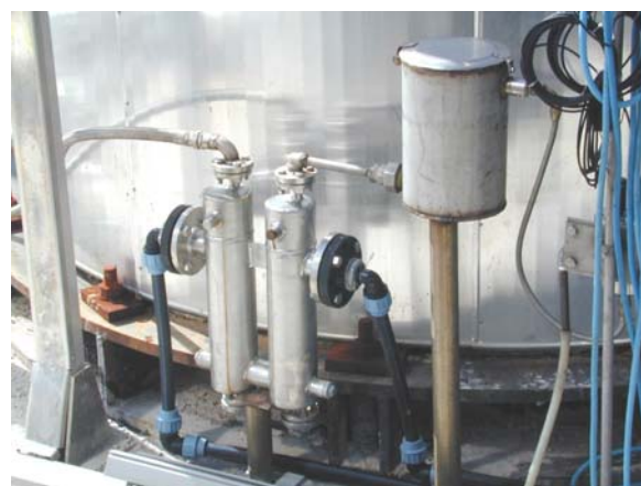
Figure 3: The cooling section on the left and the intermediate recipient for particles decantation and removal
