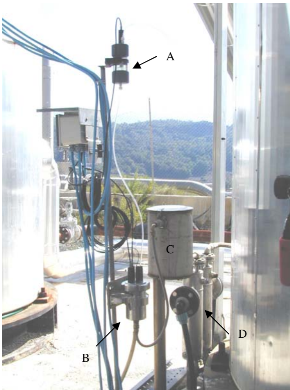
Figure 4: The entire assembly is visible. Starting from the upper left side of the picture we can see the reference electrode holder (A), the measurement electrode holder (B), the calm chamber (C) and the cooling section (D)
