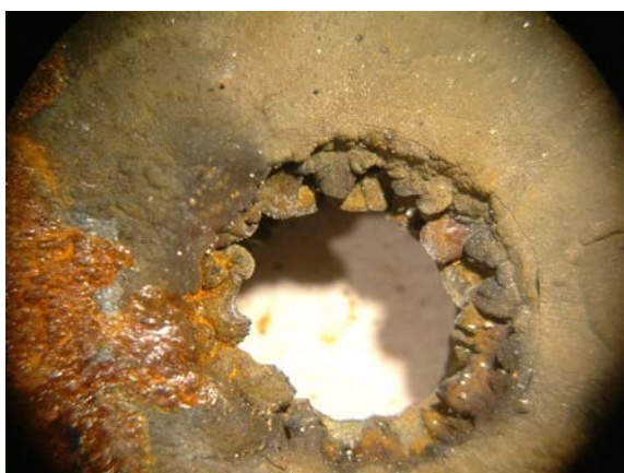
Figure 12: Orifice No. 3.2, RN-11, showing pyramid shaped scale (mostly sphalerite, & galena) where pressure was between 37 – 12 bar-g.
