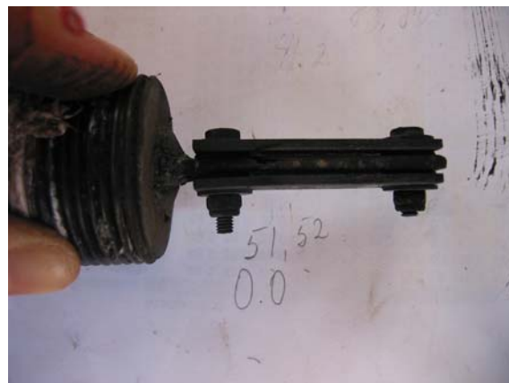
Figure 8: A set of coupons after 3 weeks experiments at location 0.0, RN-10, where pressure was between 46 – 52 bar-g. The golden scale on the coupons holder is chalcopyrite.
