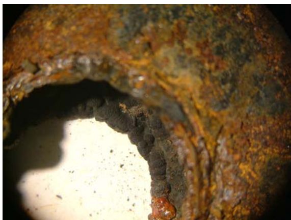
Figure 11: Orifice No. 1.4, RN-11 pressure is 14 – 5 bar-g. Black pillows are mostly amorphous silica.
