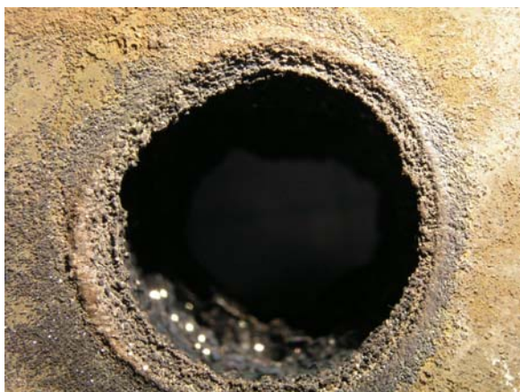
Figure 13: Orifice No. 0.0, RN-10 where pressure was between 49 – 52 bar-g. The scale is wurtzite (ZnS).
