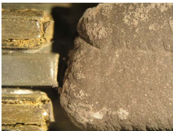
Figure 10: RN-10 coupons from location 0.0 (~50 bar-g) and 1.6 (~ 8 bar-g). Coupons at 1.6 to the left covered with scale (mostly amorphous silica).
