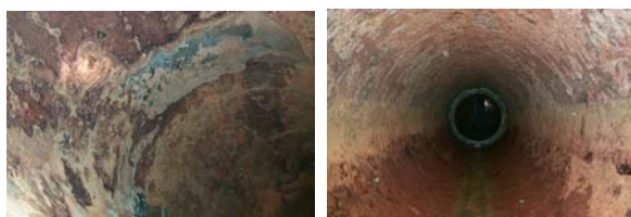
Figure 4: Hot-Side CW loss of PE and erosion at T and retained PE in straight pipe.
