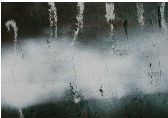
Figure 5: Vertical cracking in a longitudinal seam weld as seen after removal of corrosion products.
