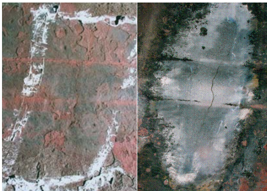
Figure 4: The typical surface of the vessel with a fine crack seen in the formed corrosion products and appearance after removal of corrosion products.
