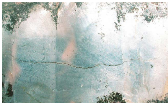
Figure 6: Horizontal crack transverse to circumferential weld C5 seen after removal of the corrosion products.
