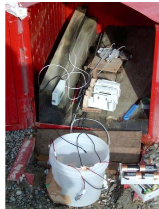
Figure 7. (a) The stations, (b) a close up view of the acoustic emission (Tekkehamam puf-puf) station.
