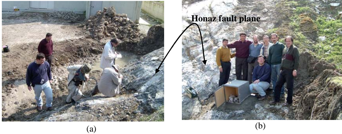
Figure 8. a: Installation of AE, TR and VR logging systems at Honaz station, b: Honaz station after the installation.
