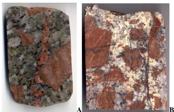
Figure 5: Examples of hydrothermally altered granite. A – Pervasive alteration which transforms primary minerals in secondary minerals but the texture is saved. Height of the sample is about 10cm. B – Vein alteration with dissolution and precipitation. Quartz deposition, brecciated granite and cataclased granite forming a hydrothermally altered zone. Height of core is about 12cm.
