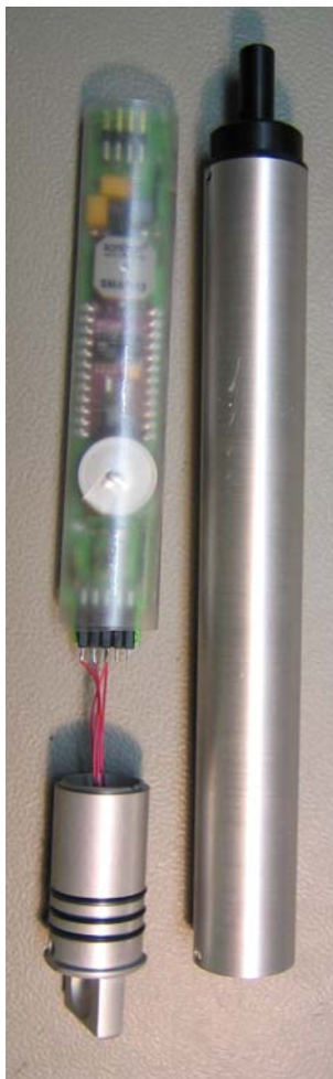
Figure 1: Sensor, electronic board and casing of the probe.
