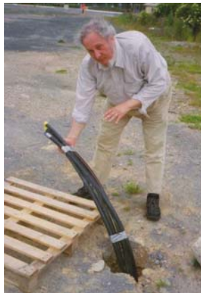
Figure 3: Test BHE at the site Wetzlar-Spilburg, ready for Thermal Response Test (photo Lund, June 2004)
