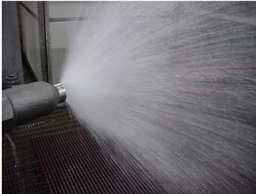
Figure 9: Sprayers Test on a Real Size Model
