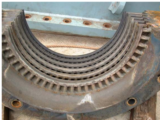
Figure 5: 1 st □ 5 th Stationary blade rows
