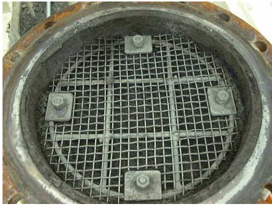
Figure 8: Mesh demister element
