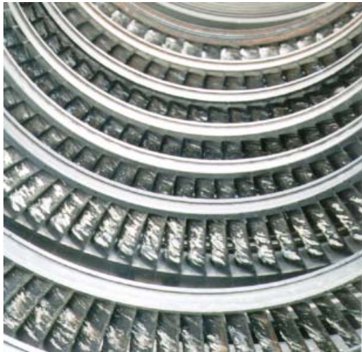
Figure 4: 1 st □ 5 th Stationary blade rows
