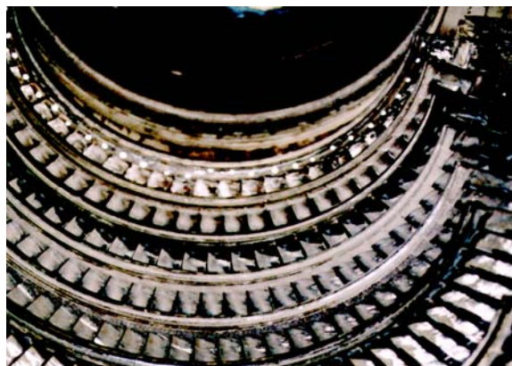
Figure 3: 1 st □ 4 th Stationary blade row
