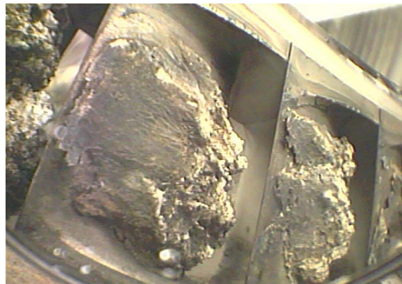
Figure 2: Scale on 1 st stage stationary blade
