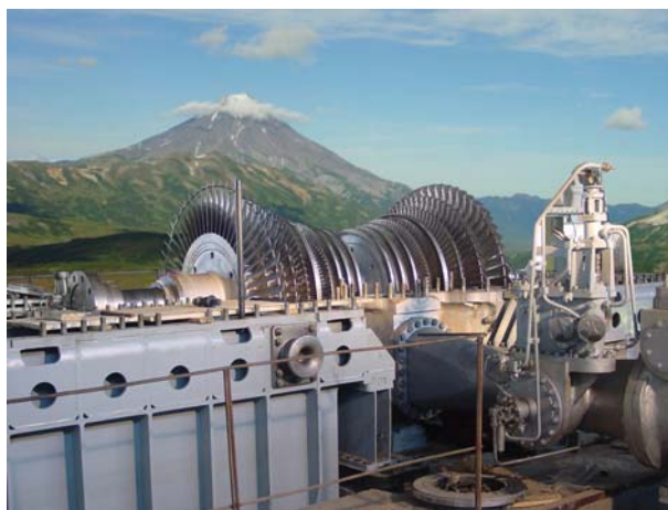
Fig. 11 25 MW steam turbine designed and manufactured by “KTZ” SC for Mutnovsky GeoPP.
