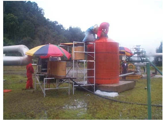
Figure 3. Photograph above show injection of 400 kilograms 1,6 naphthalene di-sulphonate (1,6-NDS) tracer in well MT2RD. The tracer is dissolved in 5000 liters of water and injected through the wing valve using 4TUT pump. Injection of the tracer solution is completed after in less than 5 minutes
