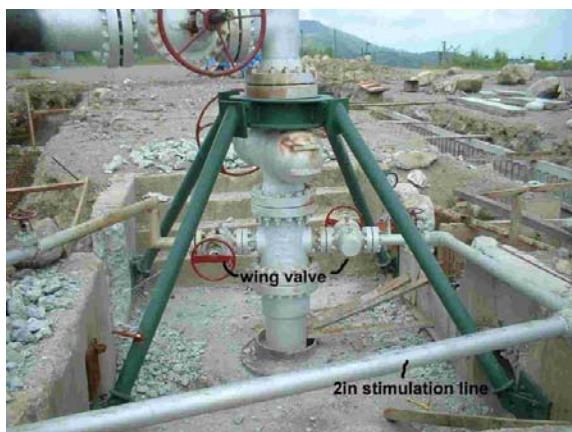
Figure 1a: Schematic diagram of a 2-in injection line set-up
