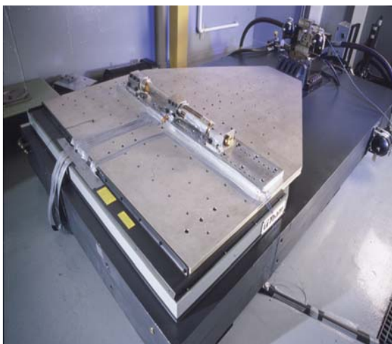
Figure 4b. Close Up of Horizontal Vibration Table Capable of 35gs
