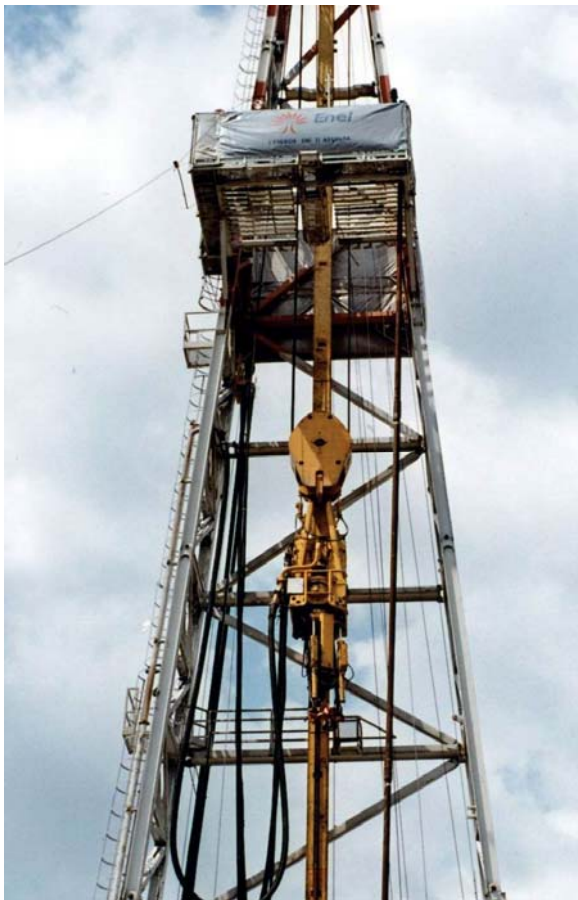
Figure 4: The top drive system in one of Enel rigs.
