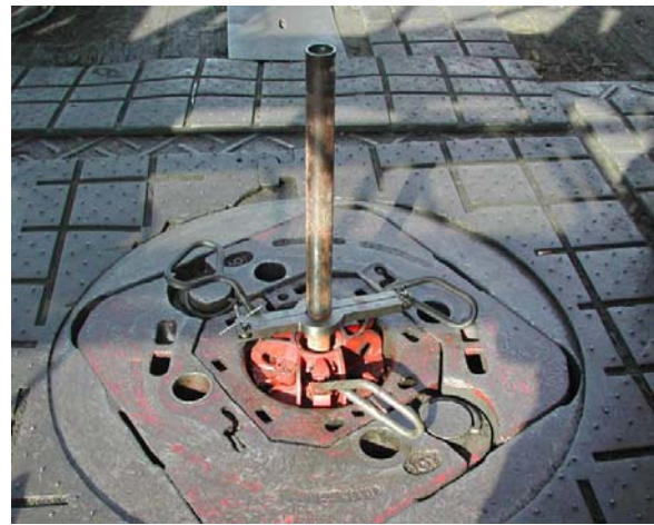
Figure 5: Surface end of the 2" down hole injection line.
