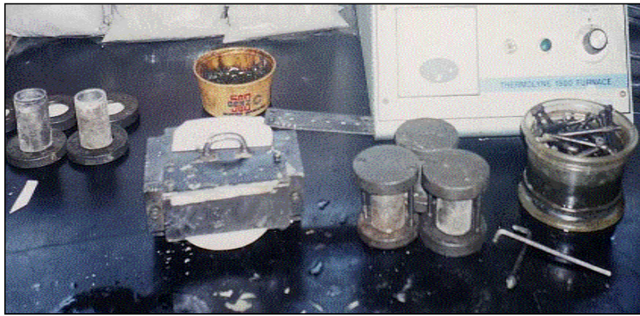
Figure 4 - The Specimens Molds (Cubic and Cylindrical Type).
