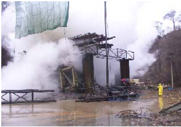
Figure 5: View of the fabricated discharge diffuser and the net (taken when Well 5R-12D was already partially quenched)
