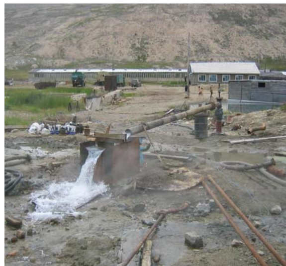
Figure 12. Flow-test installation mounted on well KU-01. The well is flowing fully open (47.5 l/s) to the V-notch container (the bath pool is seen behind the well and the greenhouse furthest away).
