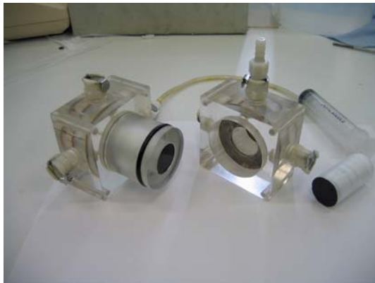
Figure 3. The equipment used for measurements of the conductivity as function of pore fluid salinity.
