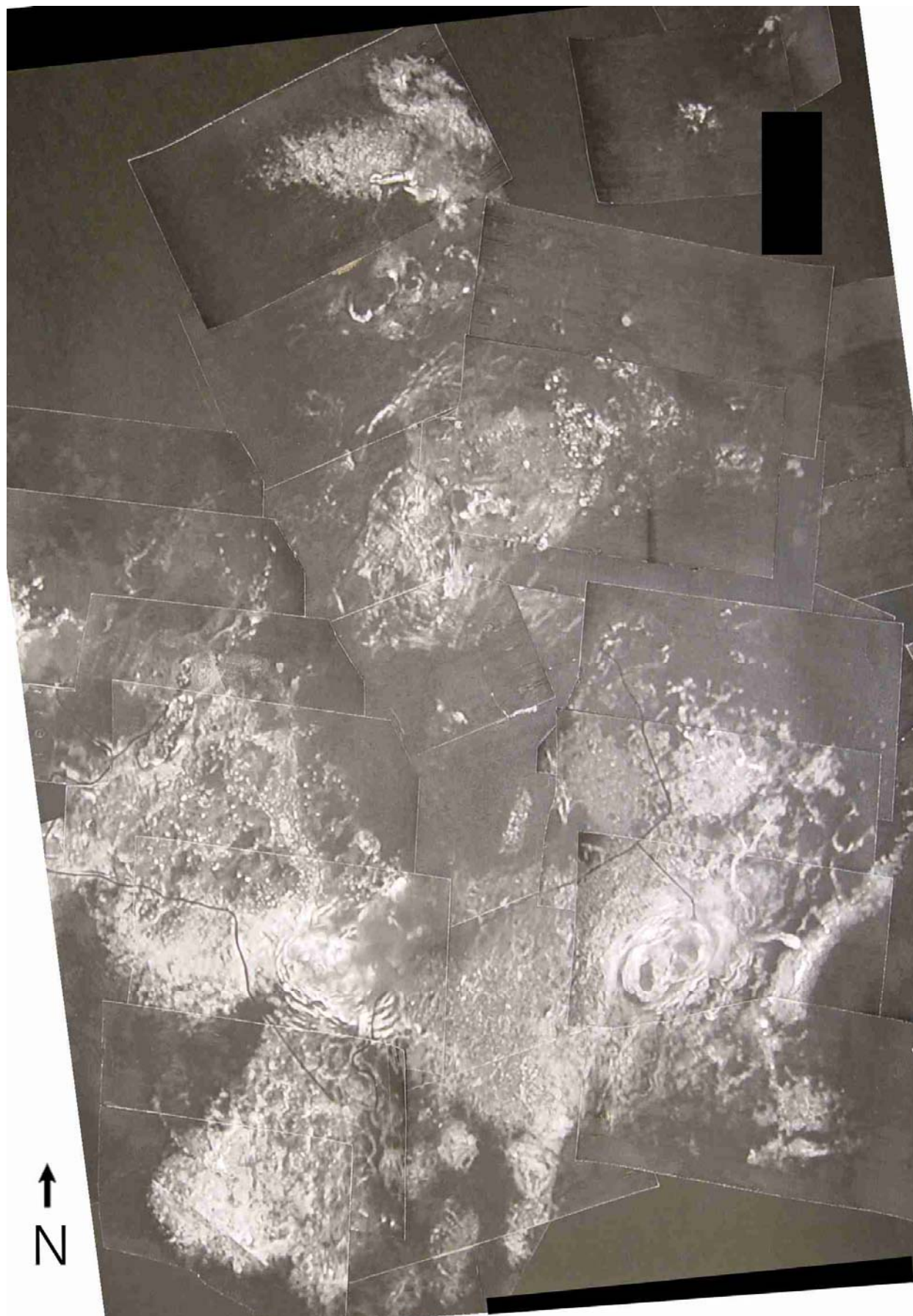
Figure 5: Thermal infrared map of Karapiti area, obtained from a mosaic of images from the 2000 IR survey, rectified to an air-photo. A 2-m wide wooden boardwalk can be seen in the image as a dark line contrasted against the anomalously hot ground.
