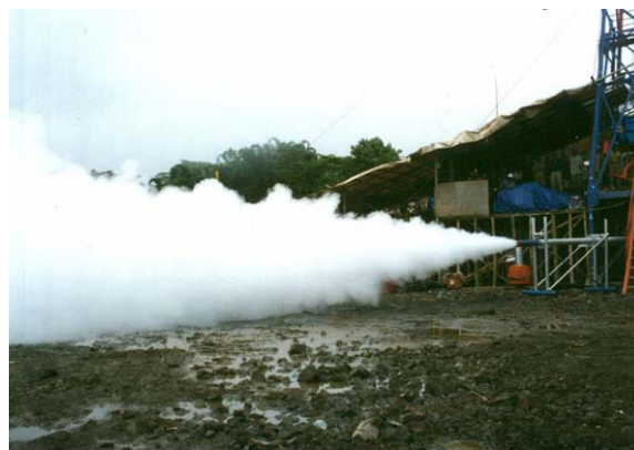
Figure 14: Photograph of the flow test of NEDO MT-2 well. It was successful. About 15 tons per hour of dry steam were stably produced at an entirely valve open state. Considering the shallower well depth of 162.35 m, the production rate is quite economical.
