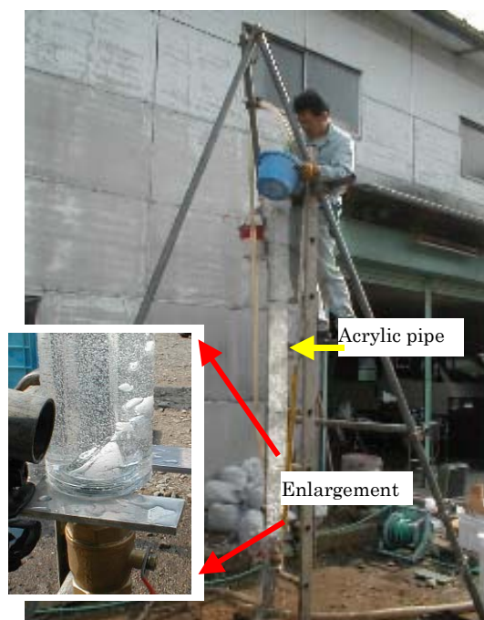
Figure 2: Preliminary frozen CO 2 injection test.
