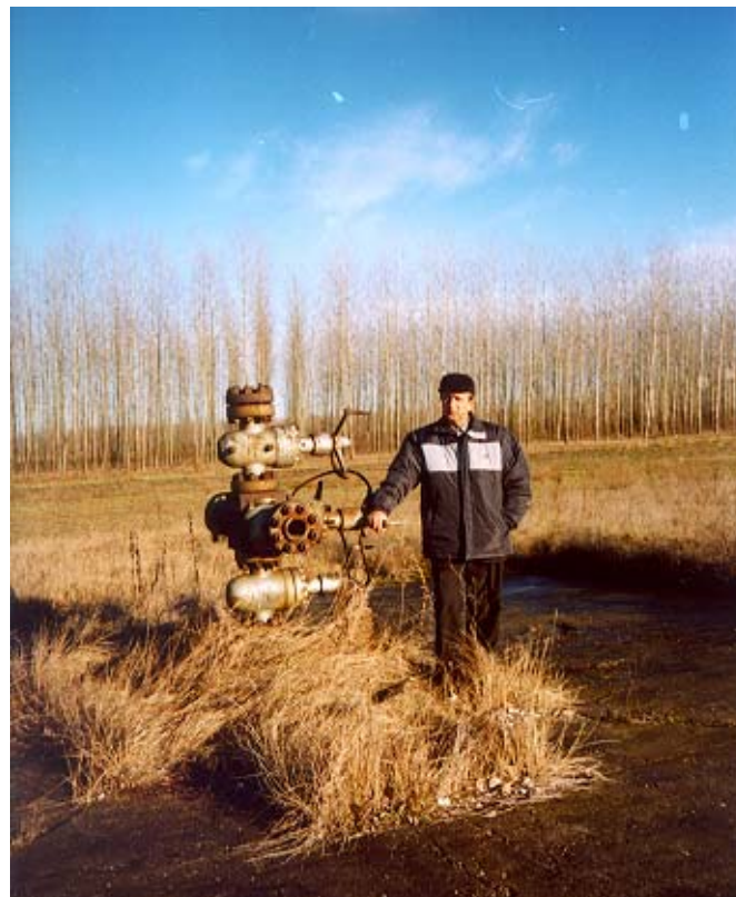
Fig 4: Well-head of abandoned CH-well X1 suitable for wet-steam production
