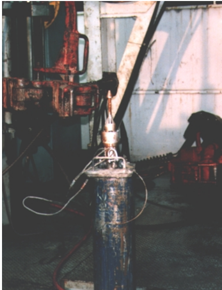
Figure 12. Prototype MWD in the actual well
