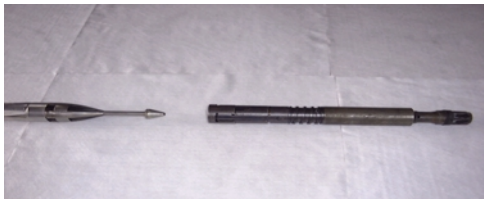
Figure 9. Releasing tool(Right) and spear point
