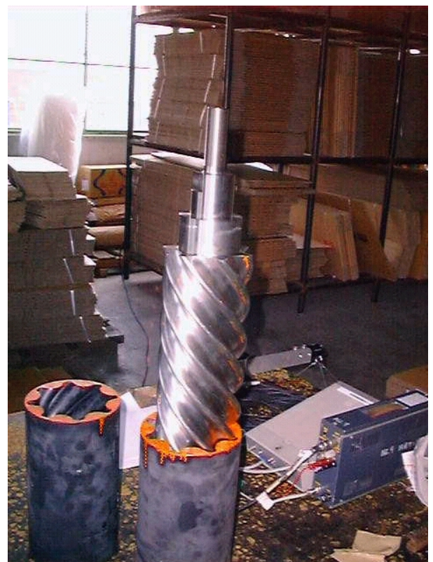
Fig.11 Rotor and stator manufactured experimentally
