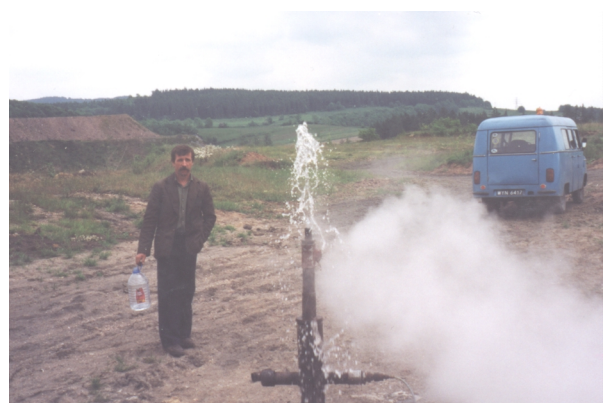
Fig. 6. Some coal mine waste heaps stay hot inside for over 50 years (here, >250^{\circ}\text{C} at depth 5 m). In the background, totally oxidised heap; Southwest Poland.
