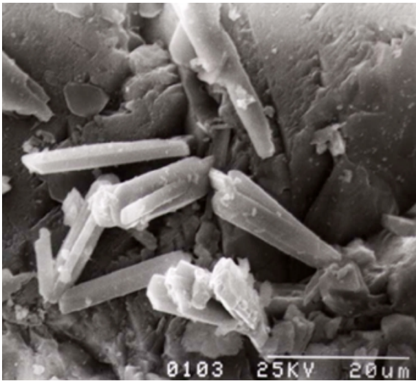
Figure 9. SEM micrograph of calc-silicate crystals on orthoclase; 400°C, 20MPa, NaCl fluid. Scale 20µm.
