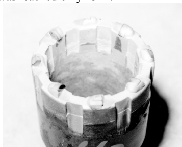
Figure 12. PDC core bit (bit No. 1 in Table 3) after the durability test. Although large amount of wear was observed at the outside cutters, wear on inside cutters was small.
