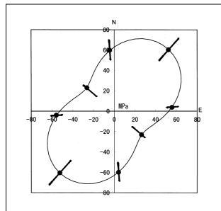
Fig.2 Estimated horizontal stresses by lab.-AE test
