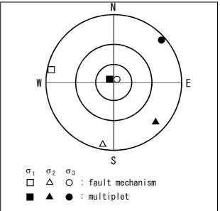
Fig. 5 Distribution of principal stresses by field AE methods (fault mechanism & multiplet) (lower hemisphere projection)
