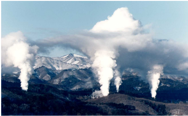
Photo 2 Well flow test at Yanaizu-Nishiyama Geothermal Power Station. Well flow steam stops rising at a certain height and trails horizontally, caused by temperature inversion that blocks diffusion upward.
