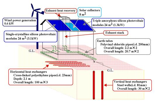
Fig. 3 Equipment design for low energy house
