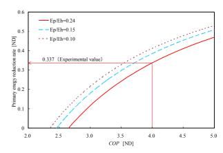
Fig. 6 Relation between *COP* of GSHP and primary energy reduction rate to typical heating
