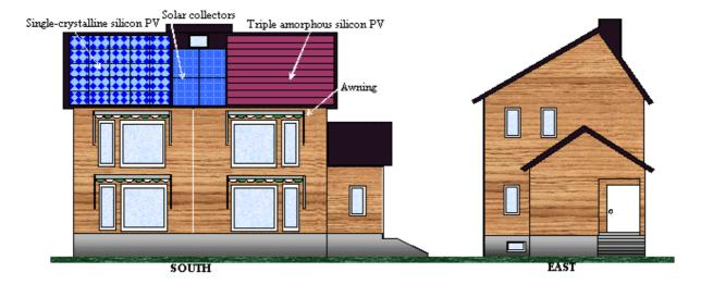
Fig. 1 Elevation of low energy house
