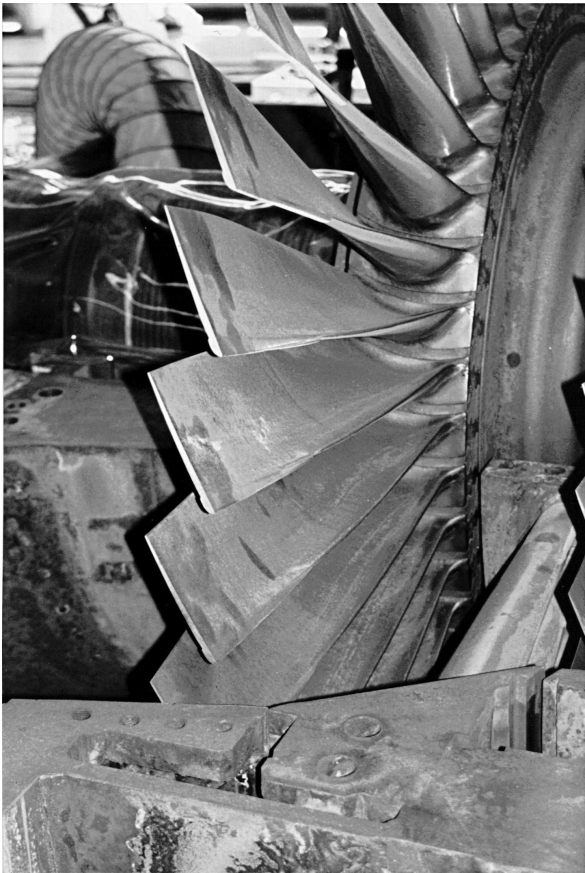
Figure 7 – Malitbog 77.5MW 3,600 rpm Turbine Blading after 18 Months Operation
