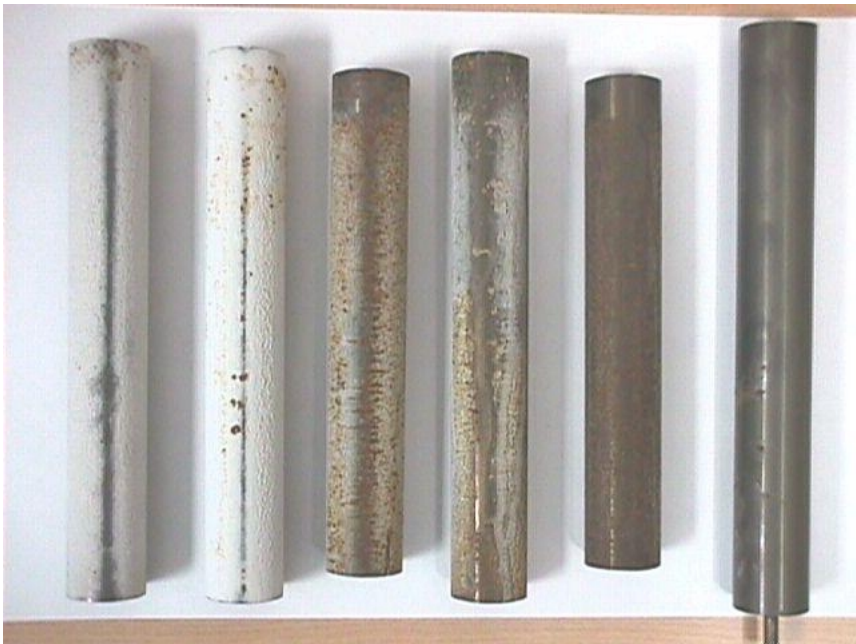
Figure 4 The six trial cylinders. From L to R, large particles, low velocity; large particles, high velocity; medium particles, low velocity; medium particles, high velocity; small particles, low velocity; small particles, high velocity
