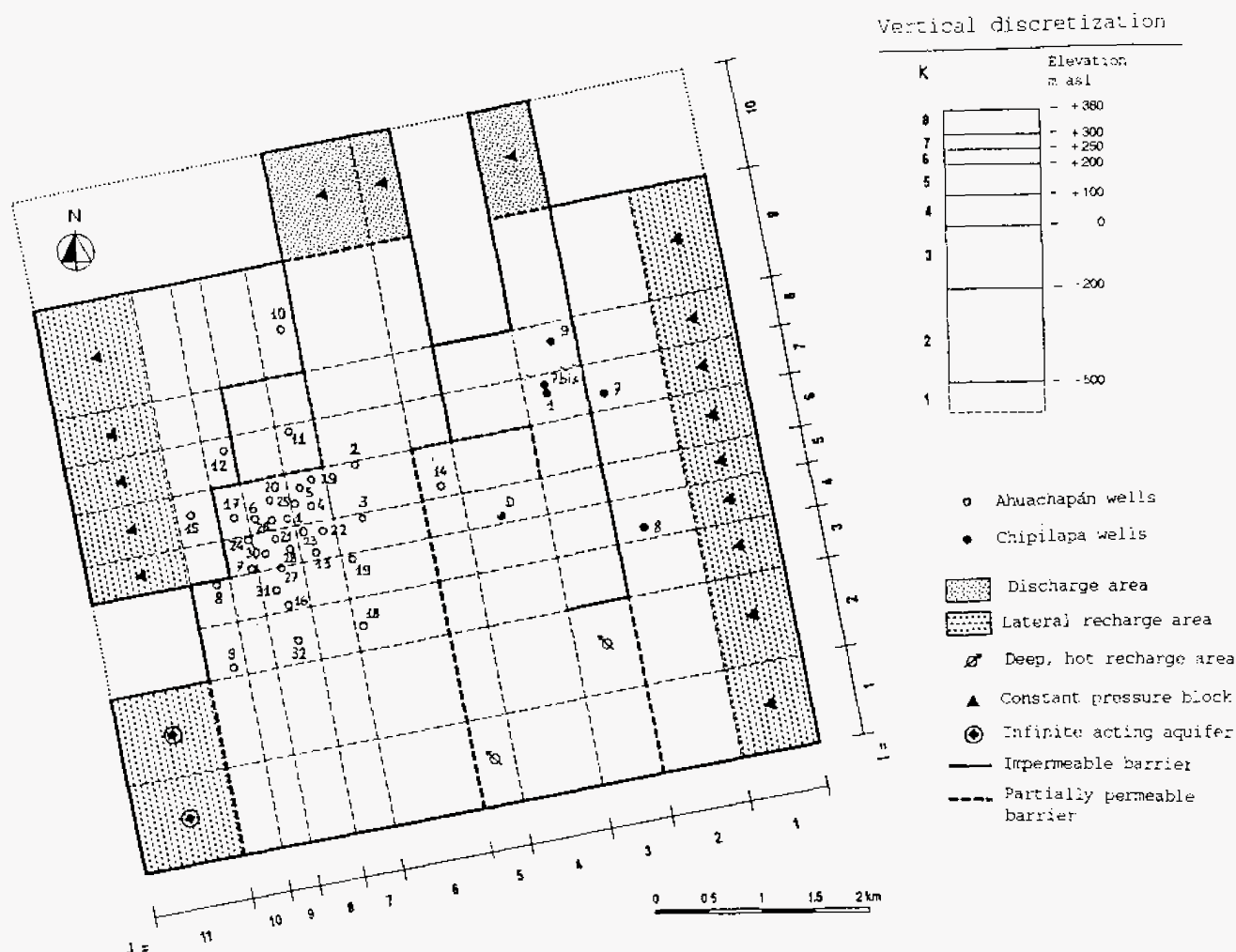
Figure 2 - Wells location, mesh geometry and model boundary conditions
