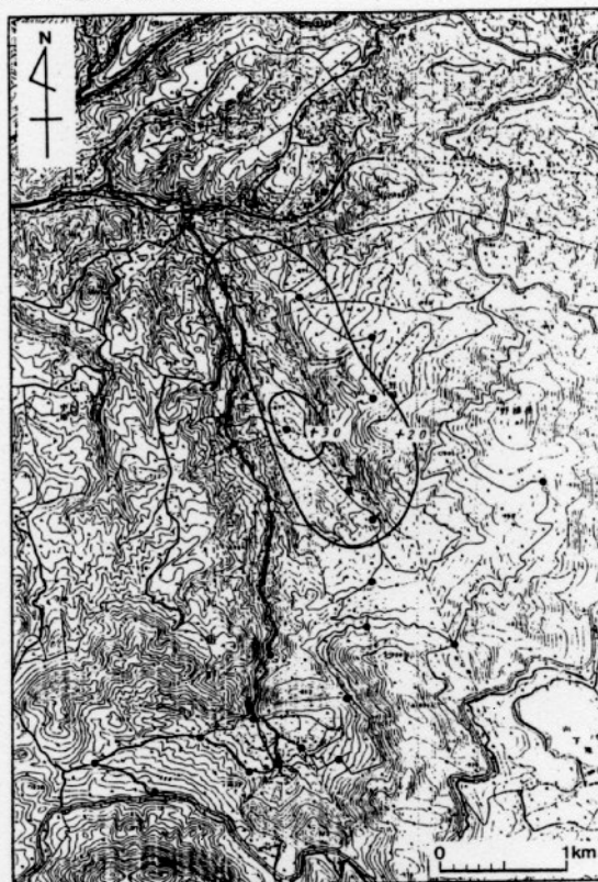
Fig. 6 Distribution of residual gravity changes in the end of the production and reinjection test. Positive anomalies up to 30 microgal are observed in the reinjection zone.
