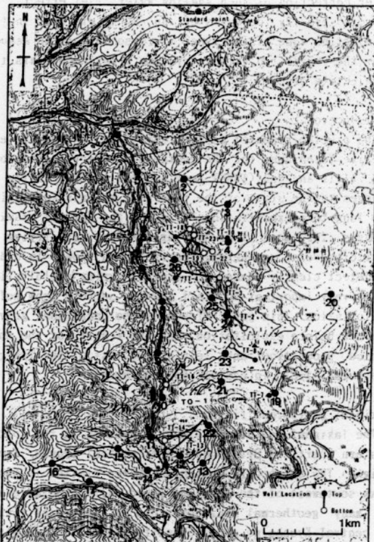
Fig.3 Distribution of production and reinjection wells (●:well head, ○:well bottom) and observation points (No.1 to 26) for the repeated gravity surveys at the Takigami geothermal field.
