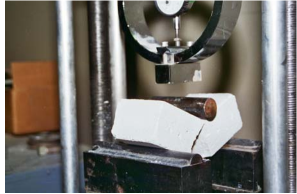
Figure 3. Flexure testing of silica-mixture bricks.
