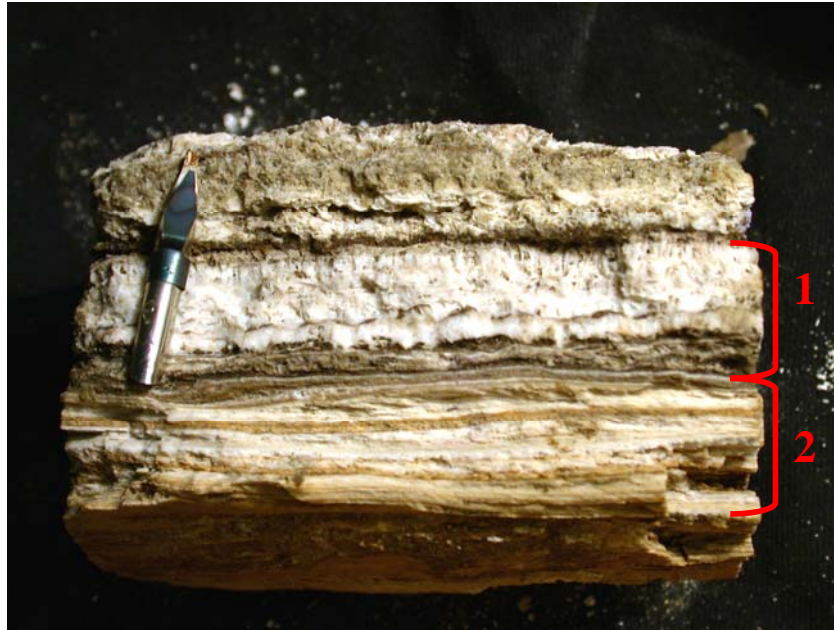
Figure 3. Types of silica structure. 1 - Cellular or spongy structure; 2 - Dense lamellar structure
