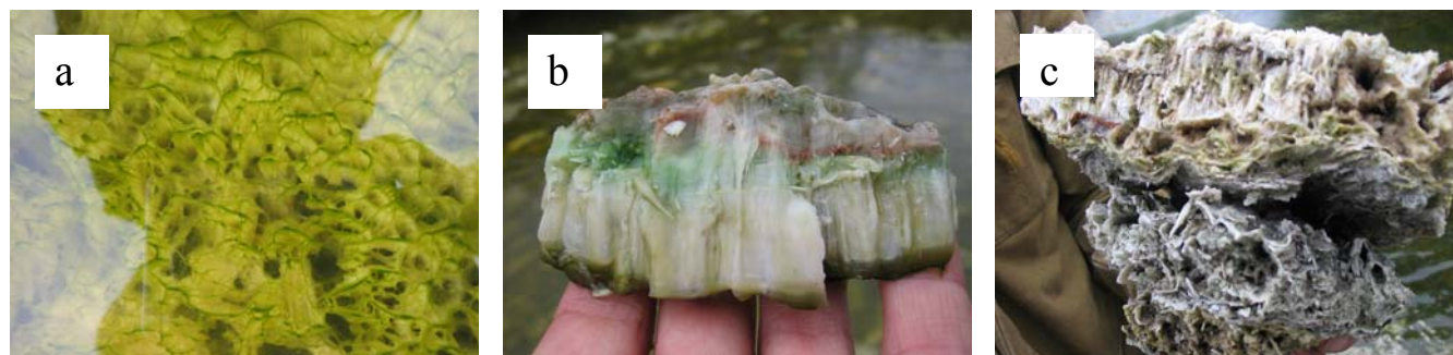
Figure 2. Artificial silica deposits: a – Thermohyllum alga; b – Silica-gel; c – Solid silica material
