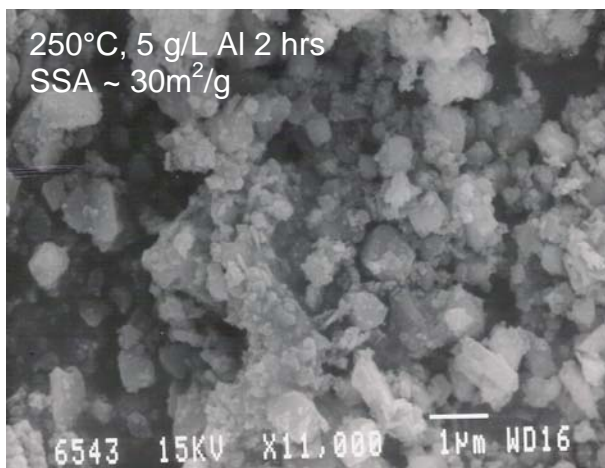
Figure 4. At 250°C, magnetite formation is far more extensive. At 10 g/L either Al or sugar, magnetite ( \text{ZnFe}_2\text{O}_4 ) and hematite are formed. If lime is not added – hematite formation is negligible. (480°F, ~400 psi)
