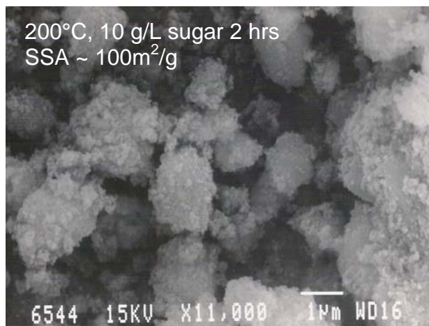
Figure 3. At 200°C, >10 g/L sugar for 2 hrs – magnetite and hematite formed from goethite. Under these conditions, magnetite can be fully substituted with Zn ( \text{ZnFe}_2\text{O}_4 ) and hematite can be substituted with Al. (390°F, ~300 psi)
