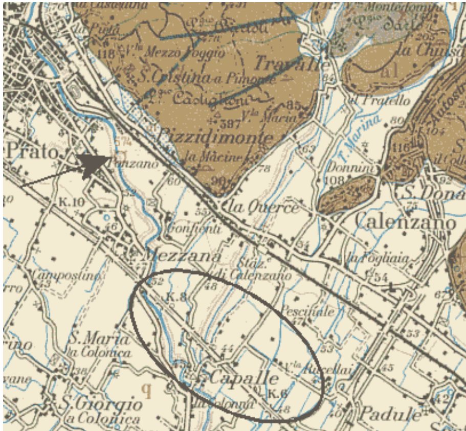
Figure 4 – Ref. Page # 106 of “Carta Geologica d’Italia”, 1/100.000. The arrow shows where a hydrocarbon exploration 574 m deep took place in the past The ellipse highlights the Campi Bisenzio zone interested in the geothermal surface exploration [4]
